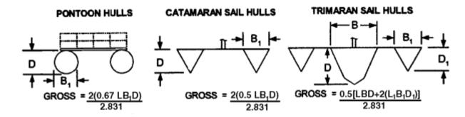
Where L is the length of the centre hull and  $L_1$  is the length of the outside hulls.
